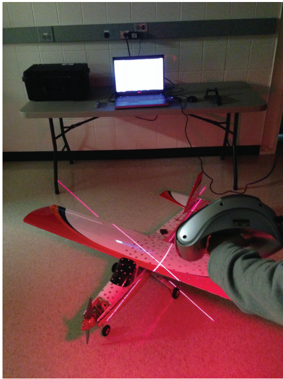
Figure 9. Scanning the top of the Avistar UAV.
