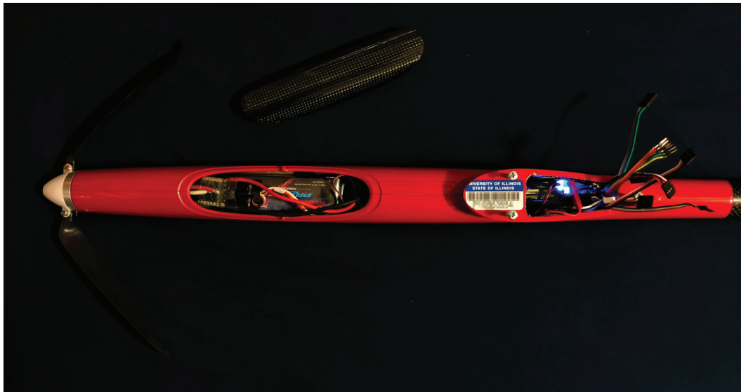
Figure 11. A photo of the top of the UIUC Solar Flyer fuselage pod showing propulsion system elements in the front of the pod and the instrumentation in the rear of the pod; note that the wires connect to the sensors and flight control actuation system located in the wing.
