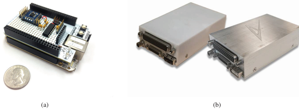
Figure 3. Data acquisition and flight control systems used as examples: (a) UIUC SDAQ and (b) AI Volo FDAQ and FC+DAQ (photo taken from AI Volo 34 ).
