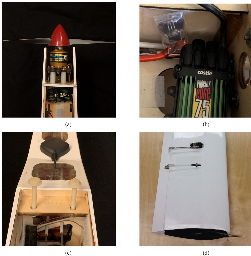
Figure 4: Key aircraft details of the as-built instrumented Great Planes Avistar Elite: (a) nose of aircraft with brushless motor, propeller, and ESC, (b) integrated Hall-effect current sensor next to the ESC, (c) rear of fuselage behind wing mounting location containing the inertial measurement unit (IMU) mounted inside and the GPS antenna on top, and (d) outer wing with aileron servo and pitot probe.
