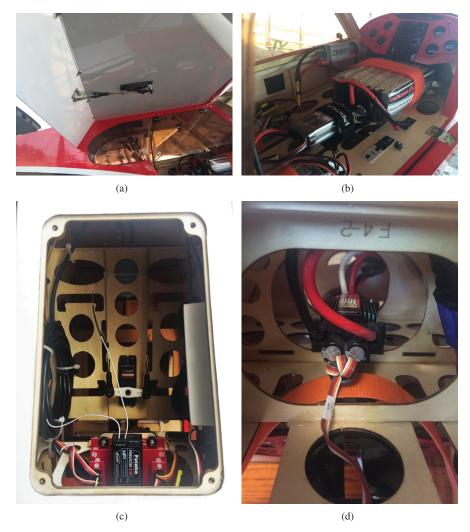
Figure 2. Aircraft construction details: (a) inner wing with flap servo, (b) top tray holding the motor, avionics, and (2) flight control batteries with the motor switch in the background, (c) rear-underside trays holding the rudder pull-pull system and servo, power distribution system with the data acquisition system mounted on the right and left, and (d) underside of the top tray holding the motor electronic speed controller (ESC).
