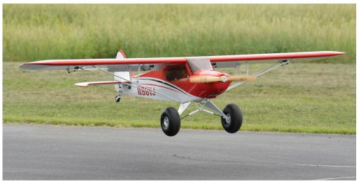
Figure 3. The 26%-scale Cub Crafters CC11-100 Sport Cub S2 during takeoff.
