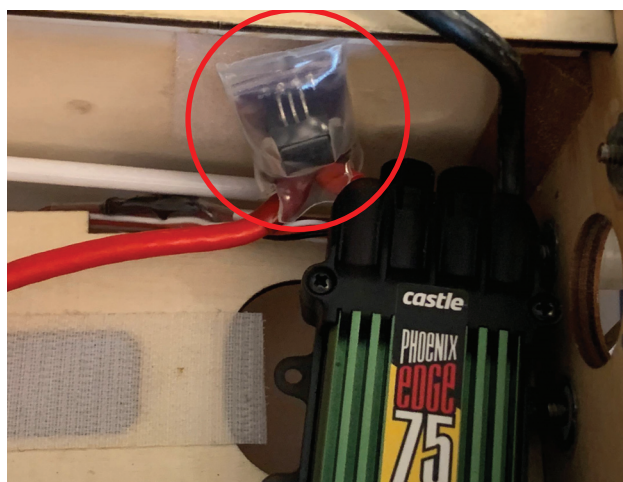
Figure 10. The integrated Hall-effect current sensor (circled in red) next to the ESC in the UIUC Avistar UAV; note that these components are situated on the battery tray with the firewall and nose of the aircraft to the right.
