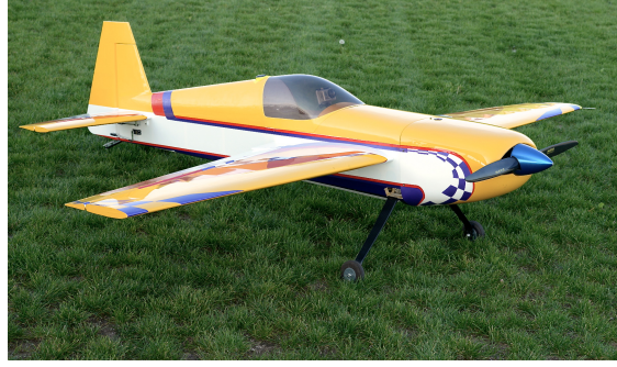
Figure 1. Photograph of the 35% scale Extra 260 UIUC Aero Testbed. 18,19
