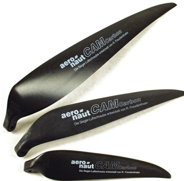
Figure 2: A photo of several Aero-Naut CAM carbon folding propeller blades (taken from Aero-Naut 8 ).
