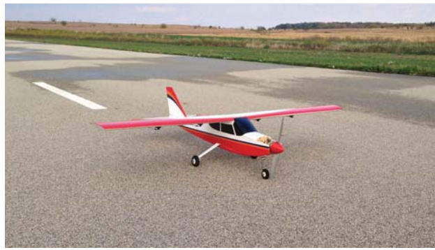
Figure 6: Flight-ready Avistar UAV.
