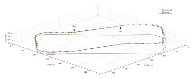
Figure 9: Comparison of aircraft path for experimental (red) and simulated flight (green) results; the airplane is plotted at 6x scale and every 2 seconds.
