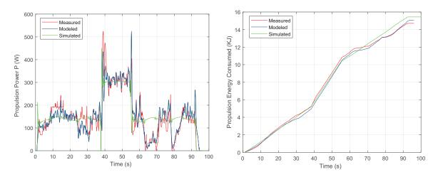
Figure 11: Comparison of (a) propulsion power and (b) energy consumed from experimental measured (red), experimental modeled (blue), and simulated (green) results using the propulsion power model assuming a non-constant lift-to-drag ratio.
