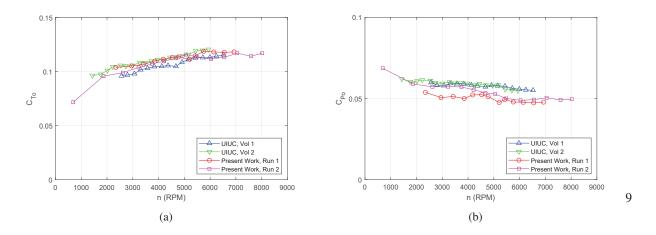
Figure 8: Comparison of static performance of the APC  $9 \times 6$  Sport propeller: (a) thrust coefficient and (b) power coefficient.
