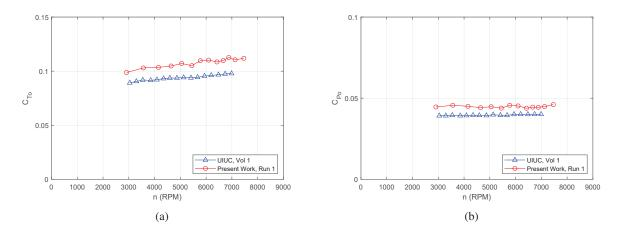
Figure 7: Comparison of static performance of the APC  $8 \times 4$  Thin Electric propeller: (a) thrust coefficient and (b) power coefficient.
