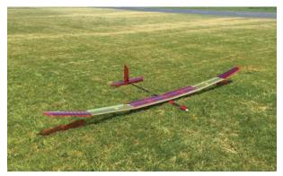
Figure 1: The baseline UIUC Solar Flyer aircraft shown without solar arrays.
