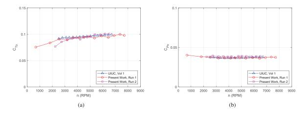
Figure 9: Comparison of static performance of the APC  $10 \times 5$  Thin Electric propeller: (a) thrust coefficient and (b) power coefficient.
