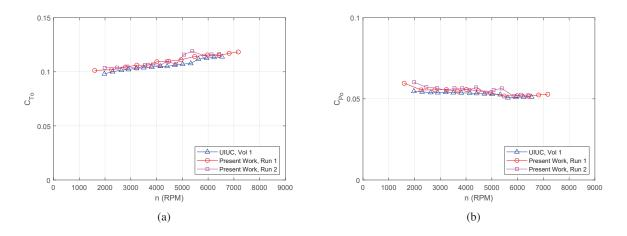
Figure 10: Comparison of static performance of the APC  $10 \times 7$  Thin Electric propeller: (a) thrust coefficient and (b) power coefficient.
