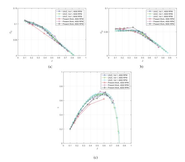
Figure 13: Comparison of advancing flow performance of the APC  $10 \times 7$  Thin Electric propeller: (a) thrust coefficient, (b) power coefficient, (c) efficiency.
