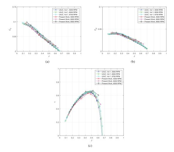
Figure 12: Comparison of advancing flow performance of the APC  $10 \times 5$  Thin Electric propeller: (a) thrust coefficient, (b) power coefficient, (c) efficiency.
