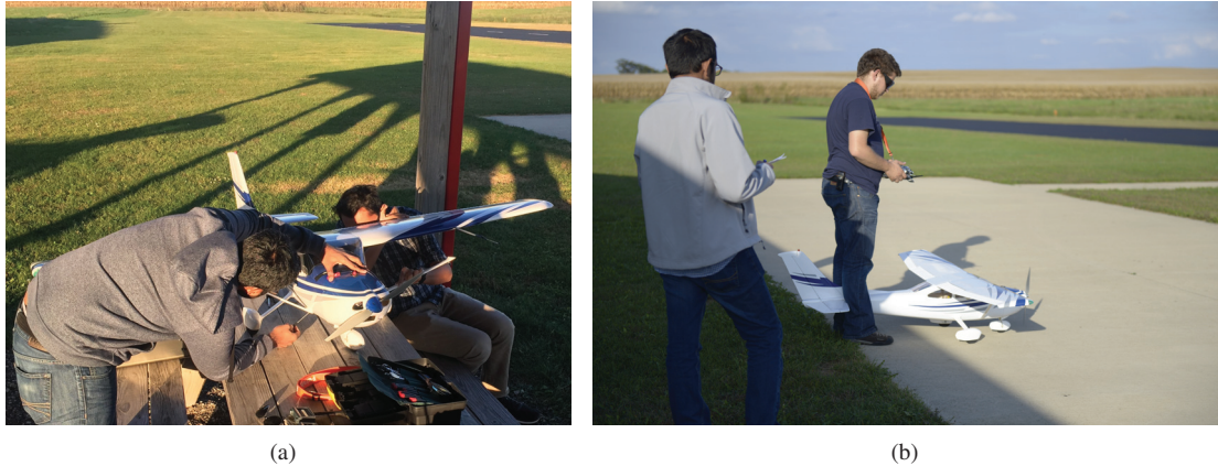
Figure 12. Preflight procedure at the field: (a) wing and strut assembly of the aircraft and (b) pre-flight motor testing.
