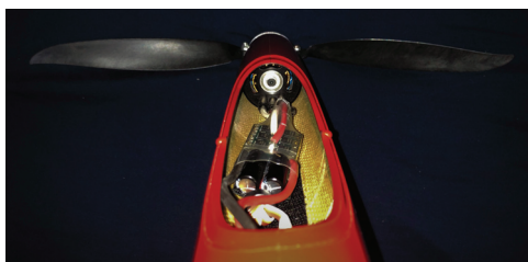
Figure 6. The propulsion system of the UIUC Solar Flyer airframe, as seen from the rear of the aircraft.
