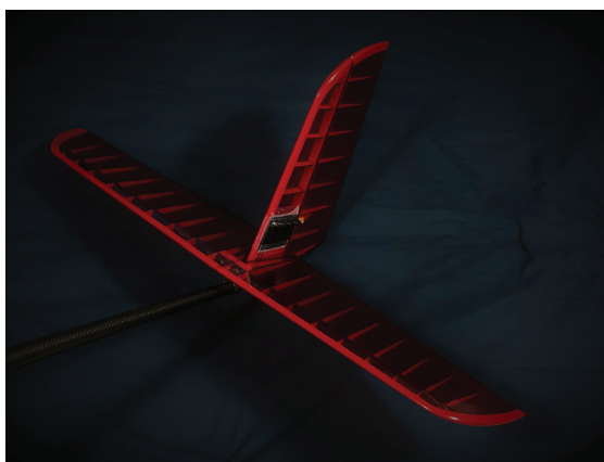
Figure 5. The tail of the UIUC Solar Flyer airframe, with a full-moving horizontal stabilizer.
