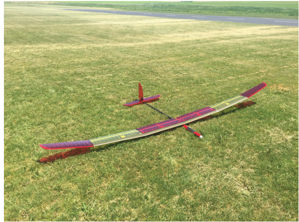
Figure 2. The F5 Models Pulsar 4.0E Pro used as the UIUC Solar Flyer airframe.
