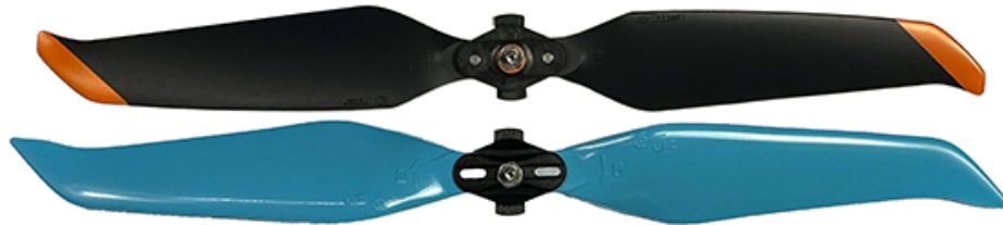
Figure 1: DJI Air 2S Low-Noise (top) and Master Airscrew Stealth (bottom) propellers.
