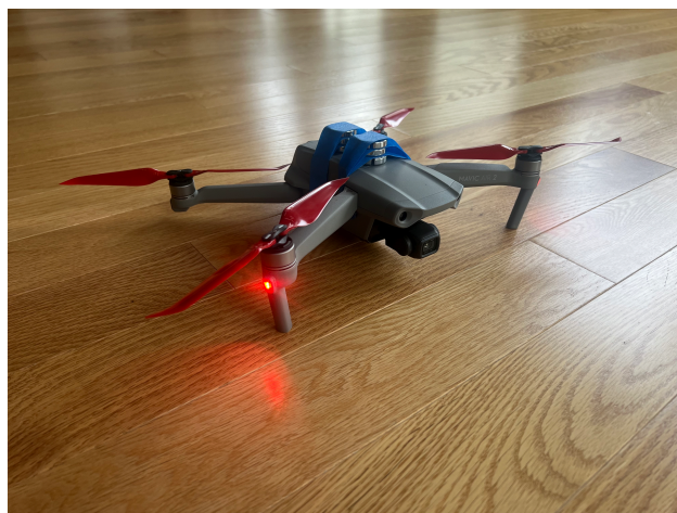
Figure 14: Example loading of additional weight on the DJI Mavic Air 2.
