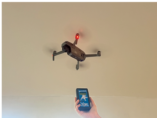
Figure 13: Measurement of propeller RPM while in flight using a handheld tachometer.
