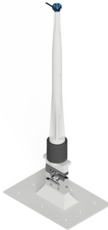
Figure 4: Isometric view of the propulsion system testing apparatus.
