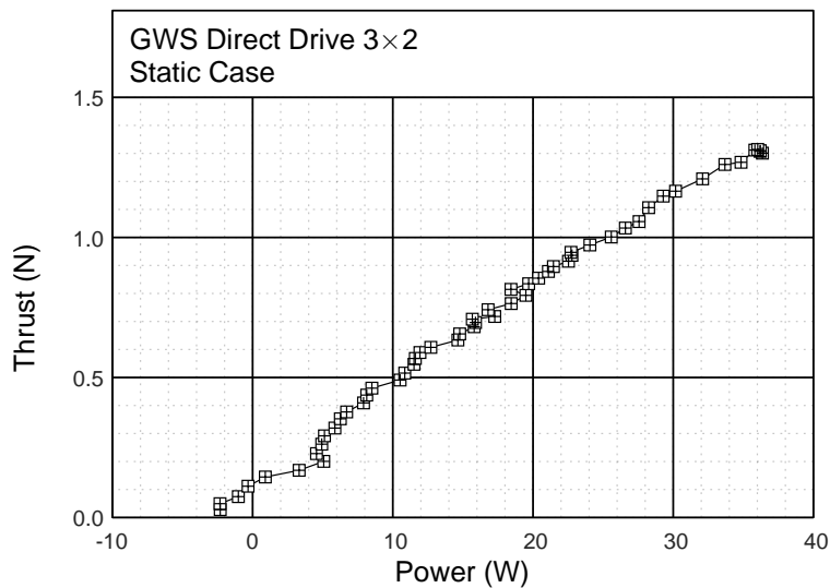
Figure 8: Plot of thrust vs electrical power for the GWS Direct Drive 3x2 propeller.
