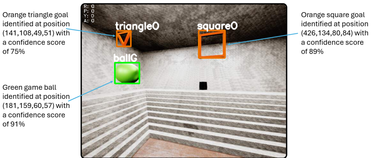
Figure 5. Image labeled by YOLOv8 perception model sent to a groundstation from simulation. Each object is defined by the center x and y of the bounding box, the bounding box's width and height, and the confidence of the model in the prediction. Image resolution and FOV intentionally mirrors the camera used onboard of a scoring vehicle in competition.
